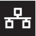
The LAN indicator light is off by default. It will turn on if you plug any device into the LAN Ethernet ports located on the back of the router. If the Wireless indicator light is off and you have a device attached:
