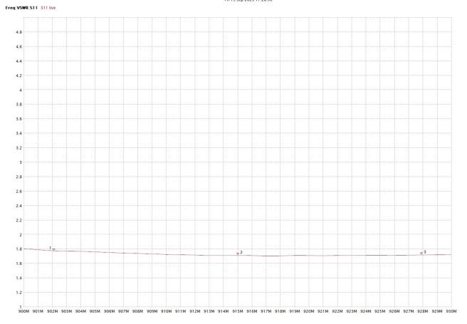
**Notes:** Antenna flex PCB measures 39x15mm and has a 100mm micro coaxial cable terminated in a u.FL connector. Lowest VSWR during testing was achieved by placing a 5mm x 1.5mm strip of foil tape approximately 3.5cm below, and parallel to, the antenna PCB element. Similar effect could also be produced by using the antenna's adhesive strip to mount the antenna approximately 3.5cm above and parallel to the device PCB to which the antenna connector will be attached.
