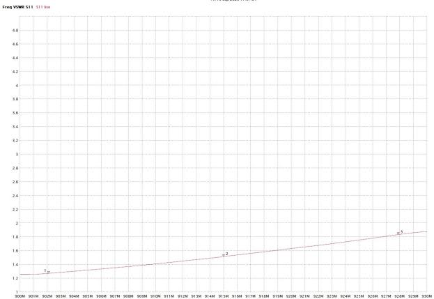
**Notes:** Antenna Flex PCB measures 100mm x 16mm and has a 50mm long micro coaxial cable terminated in a u.FL connector. Being a dipole the antenna exhibits a low VSWR and performs well regardless of orientation and without need for a ground plane.
